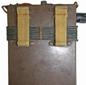
Back view of the Telesonic receiver showing the two webbing straps for carrying to the belt.
