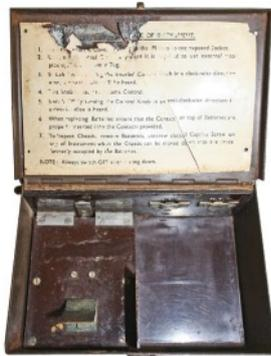
View on opened battery compartment on the top panel of Receiver Telesonic.
