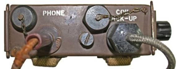
Top view of 'Receiver Telesonic' with headphones and external pick-up coil cable connected. The two dust covers are in stowed position.
